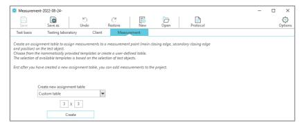
Under "Measurement", the window for creating a measuring point matrix, the assignment table, opens. There you can assign your measurements to a specific measuring point e.g., at the main or secondary closing edge and at other locations, each measured horizontally or vertically at a specific distance or height. These locations are specified in the standards and regulations for each type of test object.
