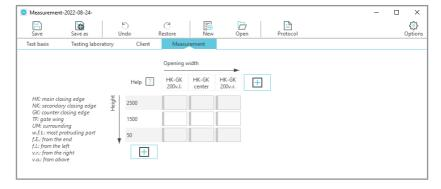
KMG-Vision suggests the horizontal and vertical locations in the assignment table according to the standard. It labels the axes if a standard has been defined beforehand.
