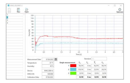
Each measurement consists of three individual measurements, from which an average is determined for:
