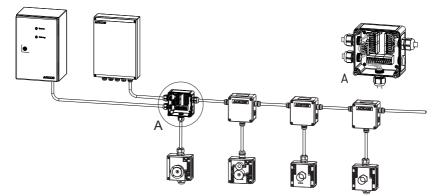
The wiring plan of the ADICOS AAB varies depending on system configuration and topology. The following procedure applies for all wiring variants.
