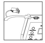
Use the connecting cable to connect the GMG-200 to the serial interface on the computer.
