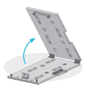
Unfold the GMG carrier plate. Ensure that it is aligned horizontally.
