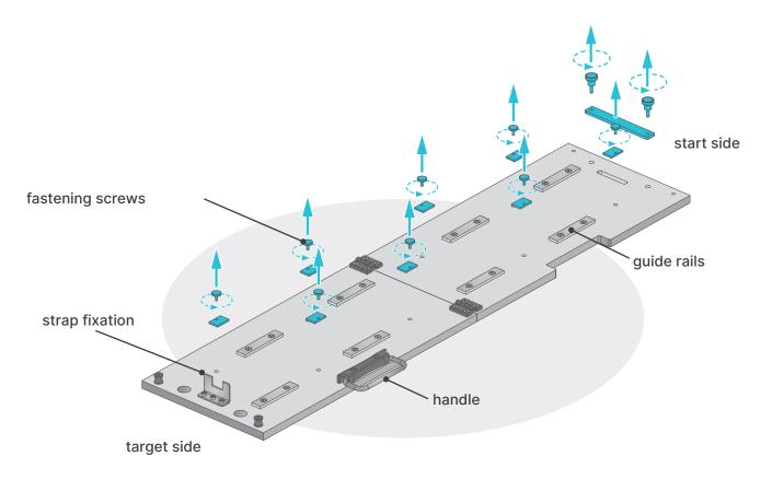
Loosen the 8 small fastening screws as well as the 2 large fastening screws on the start page.
